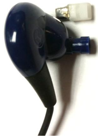
WBFK with resonator pictured with "Seashell" demonstrator earphone. A larger exit tube OD is needed to fit the tweeter assembly and allow path for woofer sound exit.
